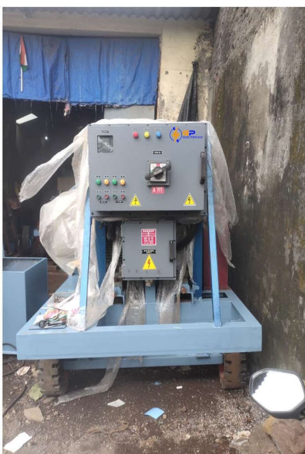
HIGH PRESSURE HYDROJET MACHINE FLAME PROOF CONTROL PANEL
